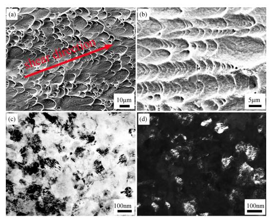
Fig. 3. (a and b) SEM images of fracture surfaces of Cu-16 at.% Al after third-pass ECAP; (c and d) bright and dark filed TEM images of the nanograins formed along the shear fracture plane.
