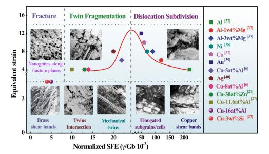
Fig. 4. Effects of SFE on the microstructures, shear fracture, grain refinement and formation of uniform structures in various fcc metals and alloys during ECAP [6,27,37–40].
