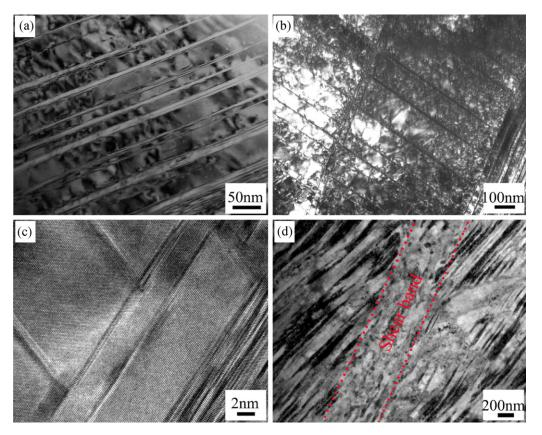
Fig. 1. Microstructures of Cu-16 at.% Al alloy after one-pass ECAP: (a) deformation twins, (b) twin intersections, (c) HRTEM images of deformation twins, stacking faults and twin intersections and (d) microscale shear bands.
