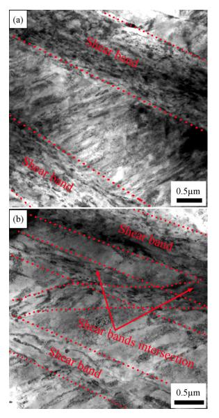
Fig. 2. Microstructures of Cu-16 at.% Al alloy after two-passes ECAP: (a) microshear bands and (b) intersections of microshear bands.
