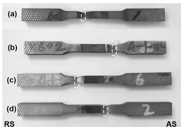
**Fig. 16** Fracture tensile samples of the joint under different cooling conditions: **a** air cooling, **b** water cooling, **c** liquid CO<sub>2</sub> + water cooling, **d** liquid CO<sub>2</sub> cooling
