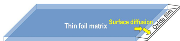
Fig. 7. Schematic map illustrating that enhanced surface diffusion yields a thicker wedge-shaped oxide film on the wall of the thin foil matrix.
